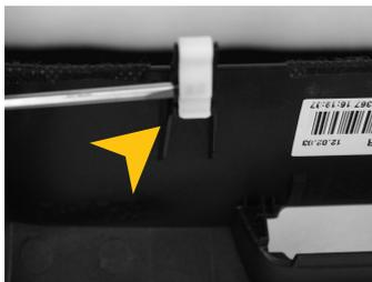
16.) Remove carefully the plastic brackets from the original radio panel and attach them at the enclosed mounting frame from the ESX device.
