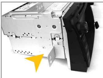
10.) Remove the metal mounting brackets on the original radio and mount them accordingly to the new ESX device.
