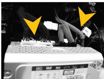
12.) Now connect the 2 original connectors of the vehicle and the included cable connectors with the ESX device (pg. 6).
