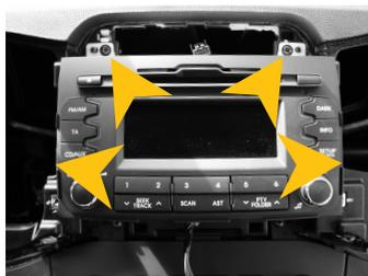
8.) Remove all 4 screw from the original radio (Phillips screw).
