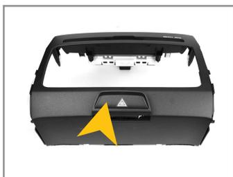
15.) Unlock the warning light switch from the original radio panel and attach it at the enclosed panel from the ESX device.
