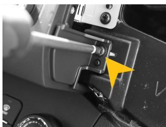
6.) Remove the right screw (each side 1) of the radio panel (Phillips screw).
