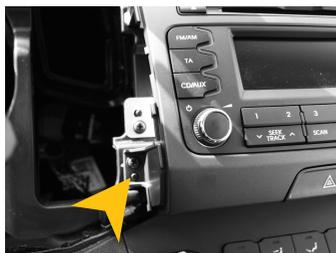
5.) Remove the left screw (each side 1) of the radio panel (Phillips screw).
