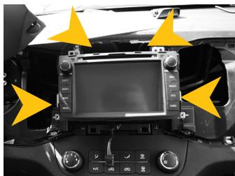
13.) Slide the unit carefully into the bay and secure it with the 4 original screws.
