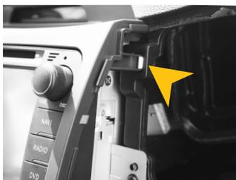
18. Now attach the enclosed panel at the vehicle's dashboard. Use therefor the 2 screws from step 5 and 6. Ensure that the plastic brackets from image 17 engage.
