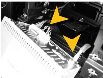
9.) Pull out the original radio from the bay and disconnect all connectors on the rear.
