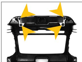
14.) Remove the 4 screws of the Airbag warning indicator at the original radio panel and secure it on the enclosed panel from the ESX device.
