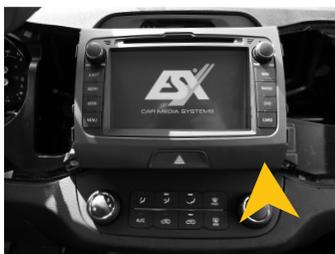
19. Before you complete the installation of the new ESX device, check its function. Please note that it may take up to 15 minutes, until a GPS signal can be received (in the open). After the successful check of the functions, re-assemble the panels in the reverse order (steps 1-4).
