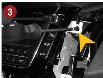
3.) Remove the four screws of the original radio.
