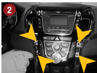
2.) Remove the four screws of the controller unit below the radio. Pull the controller unit a little out of the bay, but do not unplug the cable connections.
