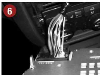
6.) Now connect all cable plugs to the new ESX device (refer to page 4-5). Plug in also all car specific cables and the antenna connector.
