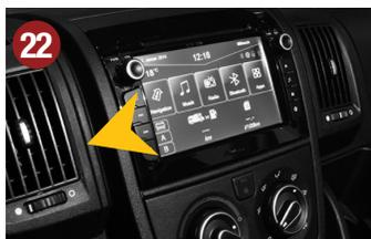
If all functions are ensured, push in the ESX device until it stops and clicks in. Then perform the re-assembly (Step 5 - 14) in reverse order.
