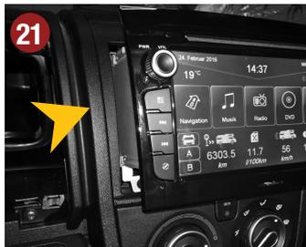
Now connect all cables and connectors of the ESX device. Slide in the ESX device carefully approx. 4/5ths into the radio bay and perform a functional test of all functions.
