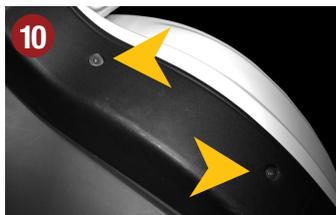
Remove the cover above the right wheel well. Loosen altogether three screws. In the picture two of them are marked.
