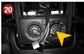
Connect the optional VNA-DUC-CAN-SET cable (See page 3) to the original connector of the vehicle. Also, connect the Antenna and the USB adaptor to the OEM connectors.
