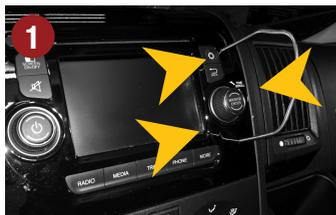
Remove the original radio with a suitable unlocking tool.
