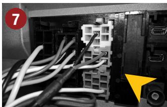
Connect the three-part mini-ISO plug of the adapter (13) directly with the ESX device.
