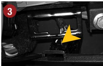
Remove the cover and unlock the connector on the left side by pressing the nose and push it out to the rear.
