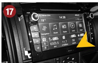
Slide the ESX device carefully into the radio bay. Before you complete the installation of the new ESX device, check its function. Please note that it may take up to 15 minutes, until a GPS signal can be received (in the open).
