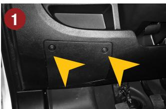
Remove the cover of the fuse box (2 x Phillips PH2).
