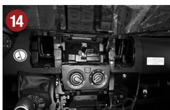
From here the installation of ESX device starts. Start from here if your car is equipped with the factory radio preparation.
