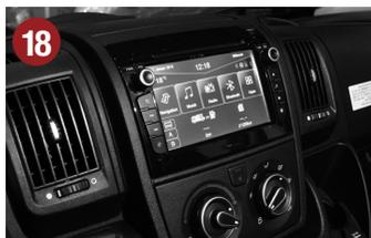
After the successful check of the functions, re-assemble the new device in the reverse order (steps no. 8 -13).
