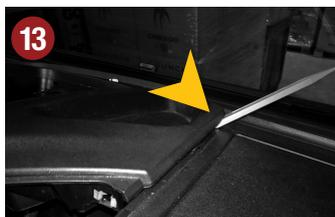
Remove the large center console screen. This is only clipped at the top at two points.
