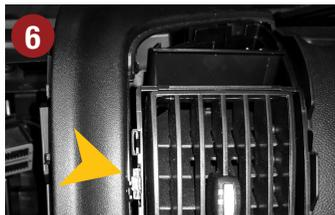
**Note:** The adjusting mechanism of vent inserts are greased!
