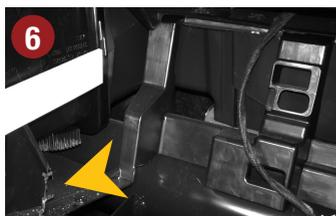
Remove the ridges inside the radio bay on both sides.
