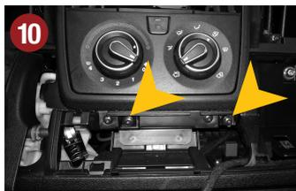
Remove the two marked screws (Torx 25, the right outside and the second from the left).
