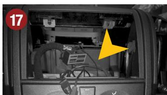
Now lay all necessary cables, for example the external microphone, USB, GPS, to the desired location. Now you can also lay additional cables such as for the rear view camera to the radio bay. Please refer to the following steps of the installation.
