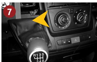
Loosen the shift boot trim. This is also just clipped, use a plastic tool and loosen it from the top.
