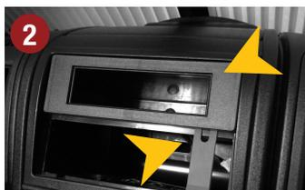
First, remove the radio and storage compartment in the dashboard. Use suitable mounting wedges.
