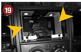
Now install the two ESX installation holders (See page 5) and fasten both with the four original screws (Torx 25) to the original mounting points.
