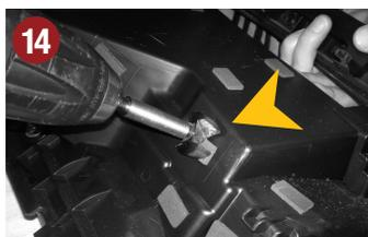
Now drill a hole (approx. 20 mm in diameter) for the USB cable on the rear of the unmounted glove box. For this, use a suitable plastic drill.
