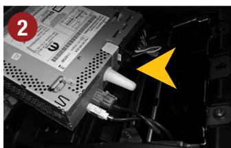
Pull out the original radio and remove all connecting cables.
