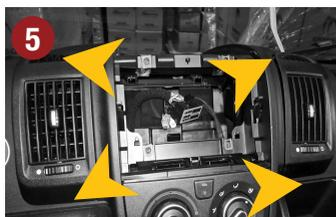
Remove the two vent inserts left and right with a suitable plastic tool. These are just clipped (see markings).
