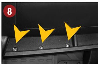
Remove the lower glove box. Loosen the three screws as marked on the image.
