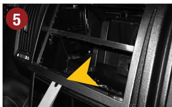
Loosen the DIN mounting frame. Use suitable mounting wedges. The pull the frame from the bay.
