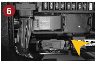
Set in the diagnostic connector MOD again, make sure that it fully locks into place.
