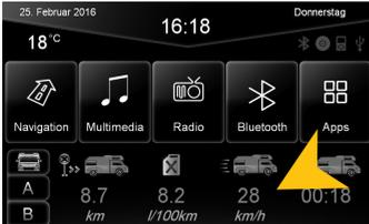
Even when there is no original radio, the CAN-Bus of the model type 290 can be connected to the ESX device to display the driving data. It is also possible to use the original steering wheel remote control and to change the vehicle settings in the „System“ menu (Apps -> System -> Option). If not available maybe an software update is necessary.
