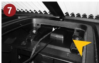
The upper storage compartment above the radio bay is perfect for the GPS antenna (12) installation.
