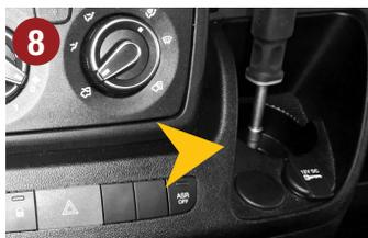
Remove the cup holder on the right inner screw (Torx 25).
