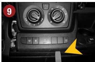
Remove the cover of the hazard switch, cigarette lighter, including cup holders unit from below with a suitable plastic tool. Then, remove all cables on the back and put the panel aside.
