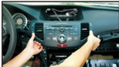
24. Install the big panel and fix with the screws
