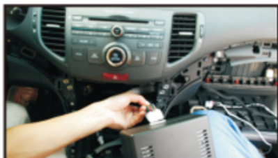
30. Connect the DVD connection wires with the DVD part
