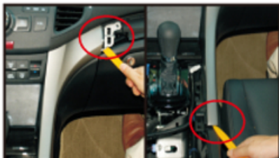
8. Pry the buckles of decorative plate with the crow plate and remove
