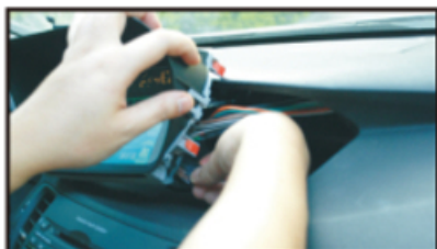
28. Connect the cables of the GPS system
