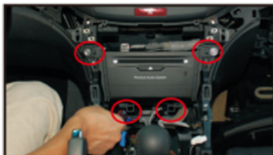
31. Fix the 4 screws on the DVD head unit
