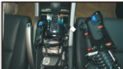
3. Remove the decorative plate and disconnect the wiring (mind the buckles and wiring)
