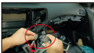
22. Connect the speaker cable with the original speaker cable
