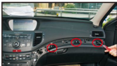
36. Install the glovebox and fix with the upper screws
