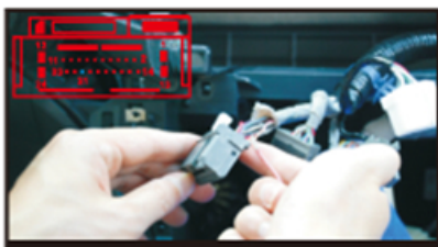
21. Connect the REMOTE cable with the 21th thin pink cable of the original system with insulating cloth
