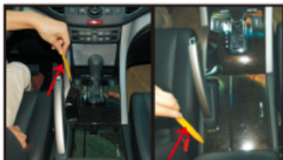
2. Pry the buckles of decorative plate with the crow plate (mind the buckles)
