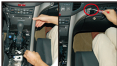
38. Install the right decorative plate and fix with screws
