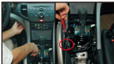
40. Install the left decorative plate and fix with the screws.
