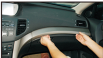
39. Install the upper decorative plate of the glovebox
