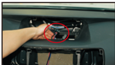
18. Take out the speaker cable as shown picture
