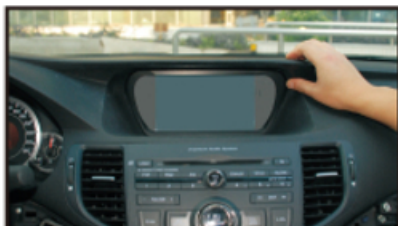
29. Install the GPS screen and connect the wires
