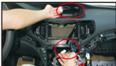
19. Install the DVD switch cable as shown picture, the upper cable should be pulled through the mantle
