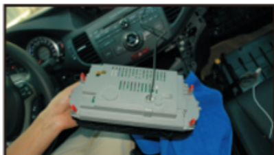
26. Install the buckles on the GPS system
