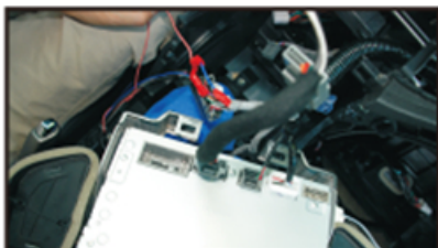
23. Connect the wires on the big panel
