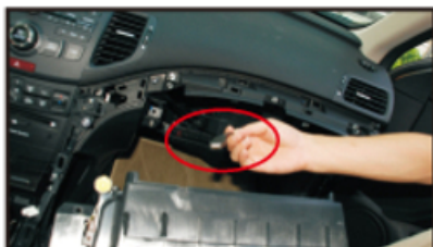
27. Install the USB cable of GPS as shown picture
