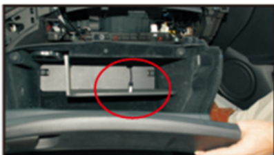
35. Put the USB connection wire in the glovebox
