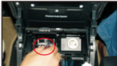
34. Fix the cigar lighter with screws and install the ash tray
