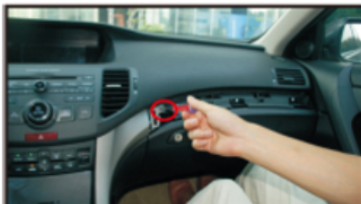
7. Pry the screws fixing the decorative board with screwdriver
