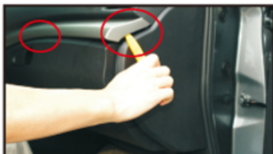
6. Pry the buckles of decorative plate with the crow plate and remove
