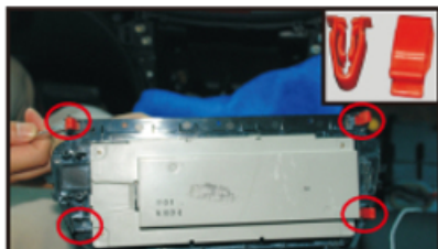
25. Take off the 4 buckles on the original screen
